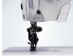
İğne transport ve ayak transport sistemi
